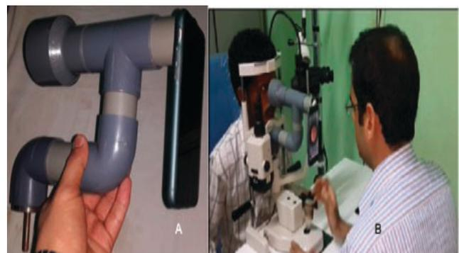
Fig 2: (A)Our instrument, (B)Instrument after mounting on slit lamp
